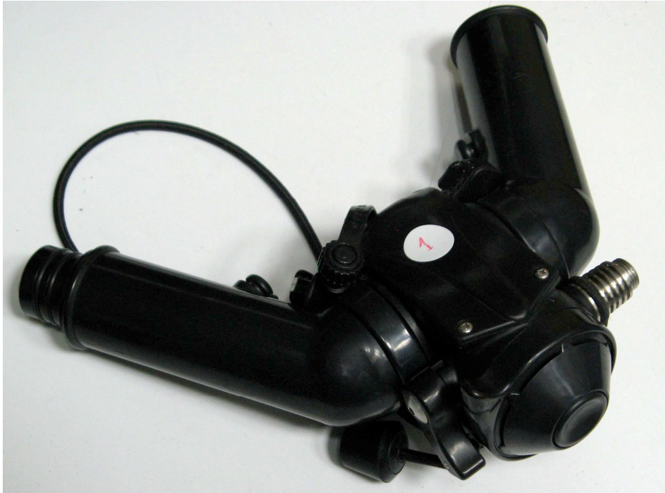
Figure 6-1. ALVBOV sample 1. Sample 2 appeared identical. CCR hoses were plugged as shown for the machine tests.
