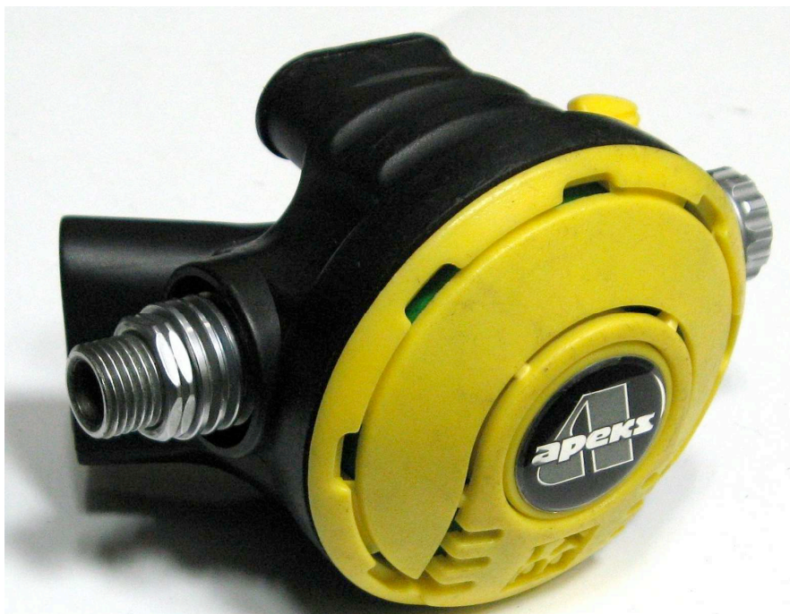
Figure 6-2. Sample of Apeks TX100 used to quantify the relevance of the flutter characteristics.
