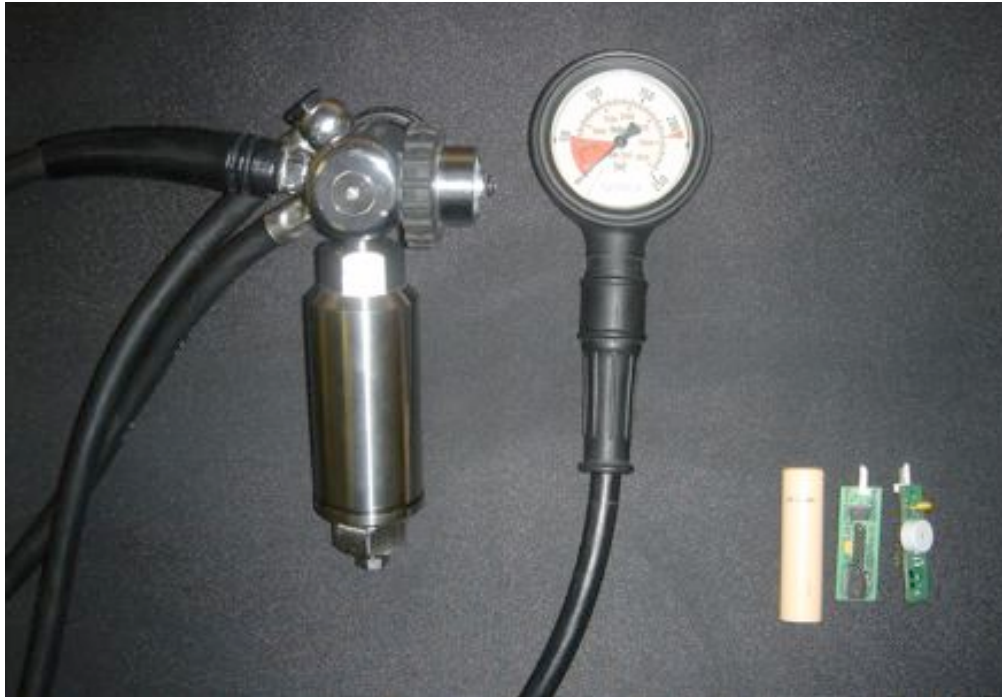
Fig 3-1: Pressure Chamber designed and fabricated for He susceptibility test, with test pcs. Shown screwed into the HP port of a regulator for first cycle tests.
